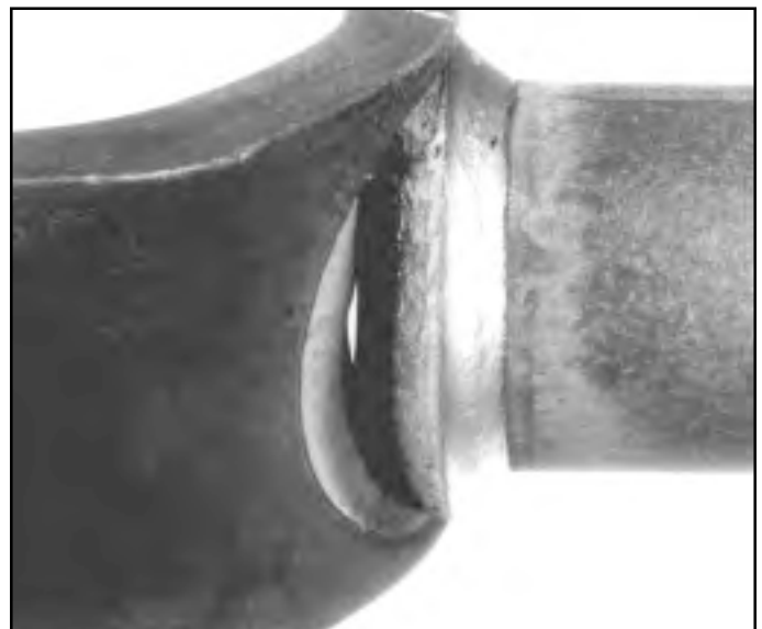
Rexnord's quality assurance program requires welded steel links to be tested for weld strength and penetration.
